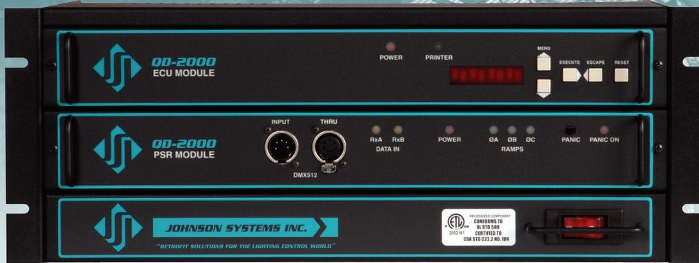
The QD-2000 is a professional retrofit electronics package designed specifically for Electro Controls (EC) Quad dimmer racks. This full-featured, state-of-the-art unit converts dual DMX inputs with protocol manager to 96 PWM and 128 DMX channels of output. Standard software includes architectural features such as DMX snapshots, scene storage, time clock, power management, auto scheduling, dimmer rack diagnostics and much more.
